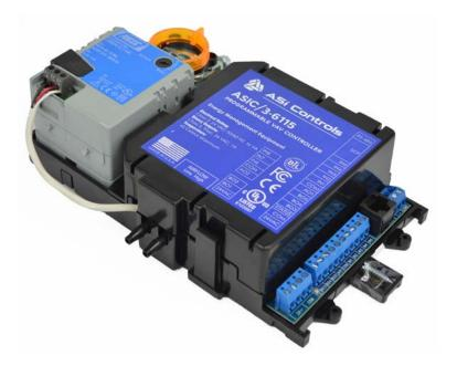
two analog outputs are used for modulated actuators, electronic pneumatic transducers, variable speed drives and other analog signal devices. The eight universal inputs counting pulses, monitoring contact closures directly, and for reading 4 to 20 mA, 0 to 5 Vdc or 0 to 10 Vdc input signals.
