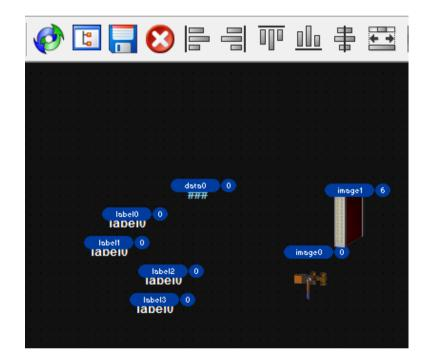
We use labels to show the voltage and the % as an example of re-using a single data tag rather than adding more tags to show voltage and %. Want to minimize data traffic between the OPC server and controller for best performance
