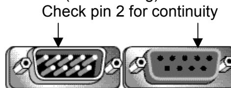
If the multi-meter shows that the pins are linked, then the cable should be fine. If the pins are not linked then you may have a NULL Modem cable. Try another cable
