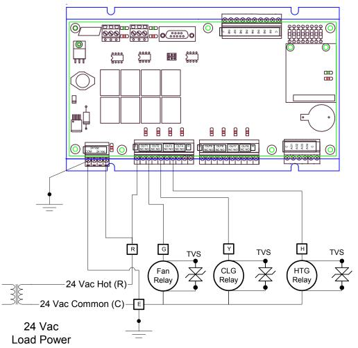
The controller power 24 Vac Hot and Common should be run directly to J8. The load power should be run separately. A TVS should be placed across each 24 Vac load relay. When a voltage spike appears across the relay coil, the TVS conducts and the excess energy is shunted to the return path. Induced currents are prevented from getting to the controller.
