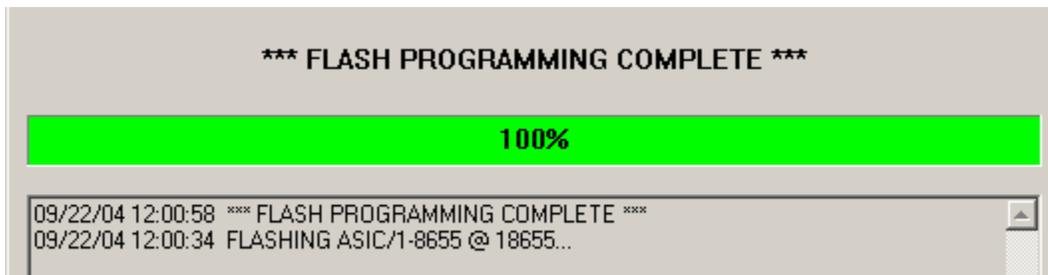
When successful, the controller goes to run mode, and the power LED comes on steady. The controller is now programmed with the new firmware. Close FlashDev by clicking the x in the upper right corner and reopen Expert.
