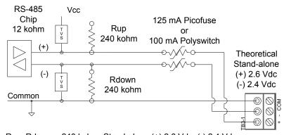
Rup, Rdown = 240 kohm Stand-alone (+) 2.6 Vdc, (-) 2.4 Vdc Typical 8655 (2.56 V, 2.24 V); 6000 (2.56 V, 2.24 V); 8x55 (2.57 V, 2.28 V)
