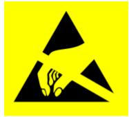
Touching the circuit board can transfer electrical charge and possibly corrupt the controller, even if the controller is not powered. It is important for anyone handling the controller to ground themselves before touching the circuit board.
