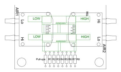
A primary airflow sensor on Input 4, and the secondary airflow sensor on Input 5 are used with a properly positioned airflow crosses to monitor primary and secondary airflow. The standard ASIC/1-8800 uses the Microswitch AWM3300 Airflow Sensor. The ASIC/1-8800-DD uses two AWM3300 airflow sensors. The airflow sensors are calibrated at zero.
