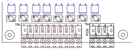
The Analog Output function may be assigned to follow the Heating Requirement or the Cooling Requirement. The Minimum and Maximum Output Voltage may be set in the configuration using ASI Expert software.
