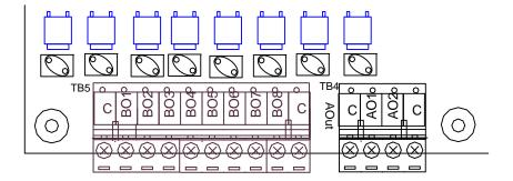
The functional assignment of the binary outputs depends on the controller personality and output mask assignments. Consult the appropriate application bulletin for the wiring and configuration details.
