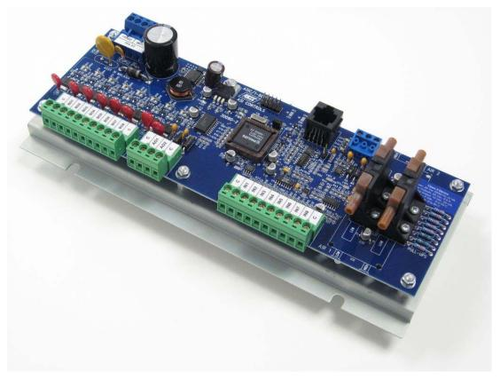
Connect the 24 Vac power. The Fan and Electric or Hot Water Heat, Primary and Secondary Dampers, and Lights are connected to triac outputs which switch the load to common as required
