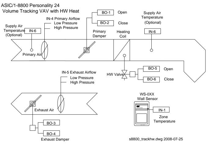
We will have to port the Volume Tracking code from the ASIC/1-8755. The primary damper is a simple VAV personality. The 8755 is built on top of 8055.
