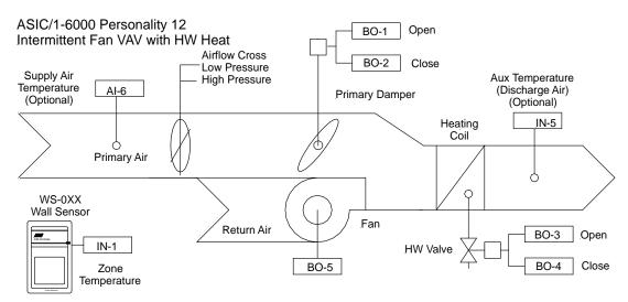
The ASIC/1-8800 is preprogrammed with different personalities for fan-powered parallel VAV system with intermittent fan.
