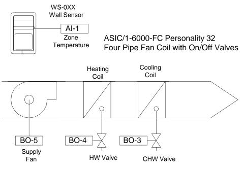
Two new personalities, 31, 2-pipe On/Off Fan Coil and 32, 4-pipe On/Off Fan Coil have been implemented for simple fan coil applications
