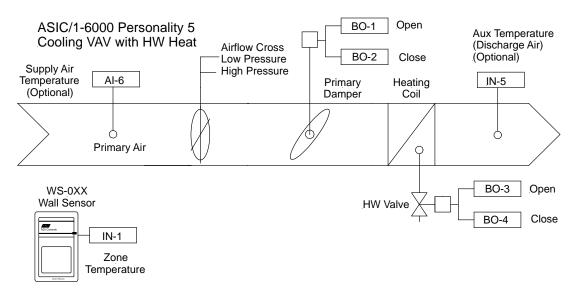
The ASIC/1-8800 is preprogrammed with different personalities for single duct cooling VAV terminals. The Zone Temperature is compared with the Active Heating and Cooling Temperature Setpoints.
