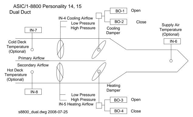
The ASIC/1-8800 is preprogrammed with two personalities for dual duct VAV system with or without blending.
