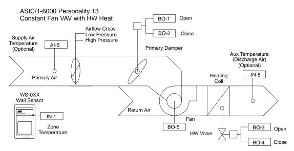
The ASIC/1-8800 is preprogrammed with different personalities for fan-powered series VAV terminals with constant fan.
