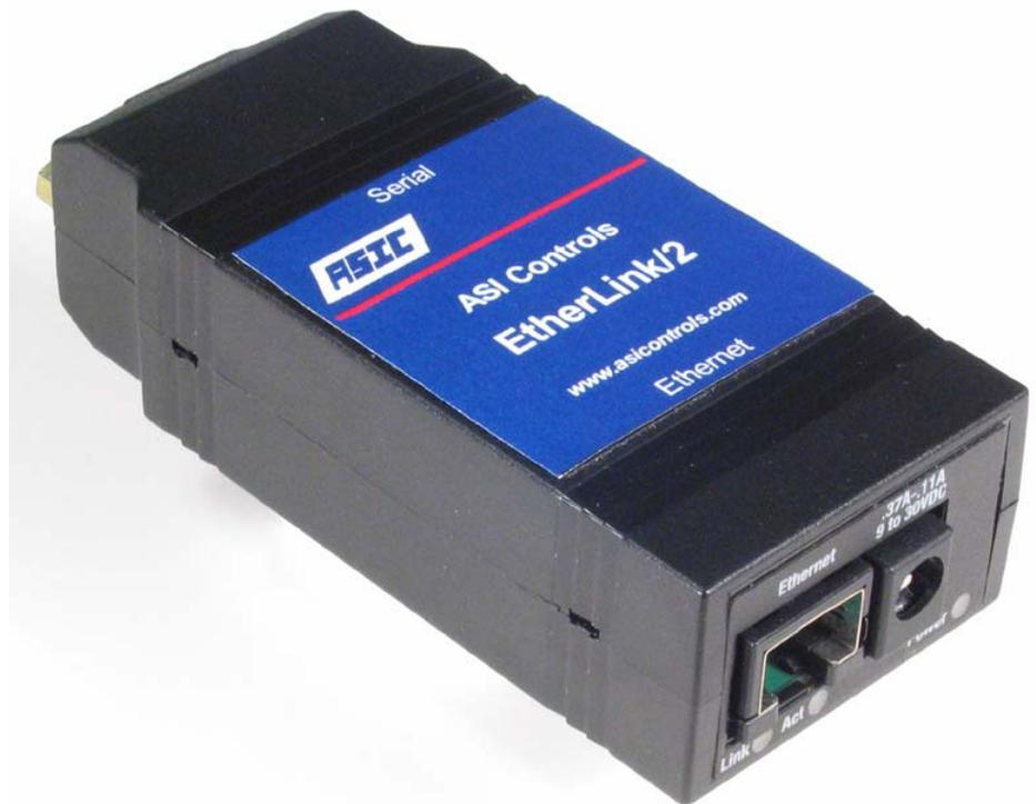
The ASI EtherLink/2 can be the primary access to the ASI network of controllers. You can connect to the system bus of an ASIC/2-7540 or ASIC/2-8540 controller using either RS-232 or RS-485 connections. You can also connect to a network of ASIC/1-8655 or ASIC/1-6000 controllers using the EtherLink/2 RS-485 cable.
